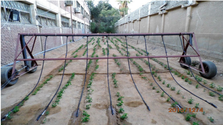
Fig. 6 First use of linear mobile drip irrigation on a pea field in Egypt in 2016. Photograph was taken in December 2015 in the research field of Irrigation Systems Engineering Department, Faculty of Agricultural Engineering, Al-Azhar University, Nasr City, Cairo, Egypt [15]
