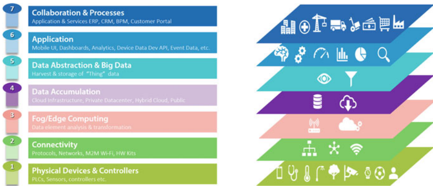
Fig. 1.3 IoT reference model by IoTWF
