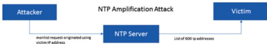
Fig. 10.1 NTP amplification attack
