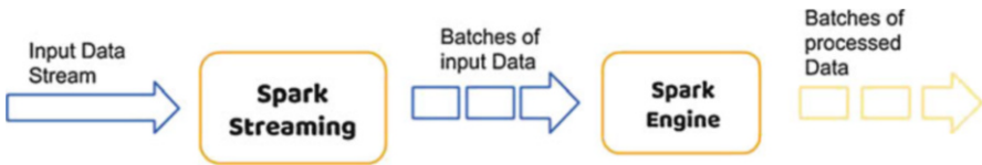
Fig. 6.19 Spark Streaming functionality
