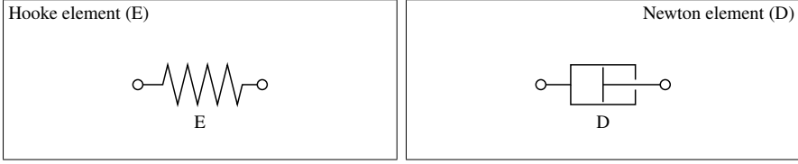
Fig. 1.2 Basic elements of rheological models used to reproduce viscoelastic material behavior
