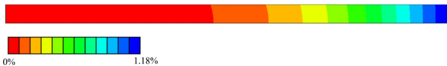
Fig. 10.9 Numerical prediction of the moisture profile of XNR 6852-1 after 24 hours of ageing. Upper bar represents one quarter of the adhesive layer while the lower bar represents a colour coded scale of the predicted moisture uptake
