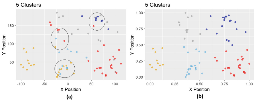
Fig. 3. Example of data clustering: (a) Original data clustering with overlapping and (b) Normalization + KNN data clustering.
