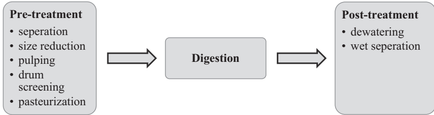
Fig. 6.2 Unit processes of biogas production from MSW
