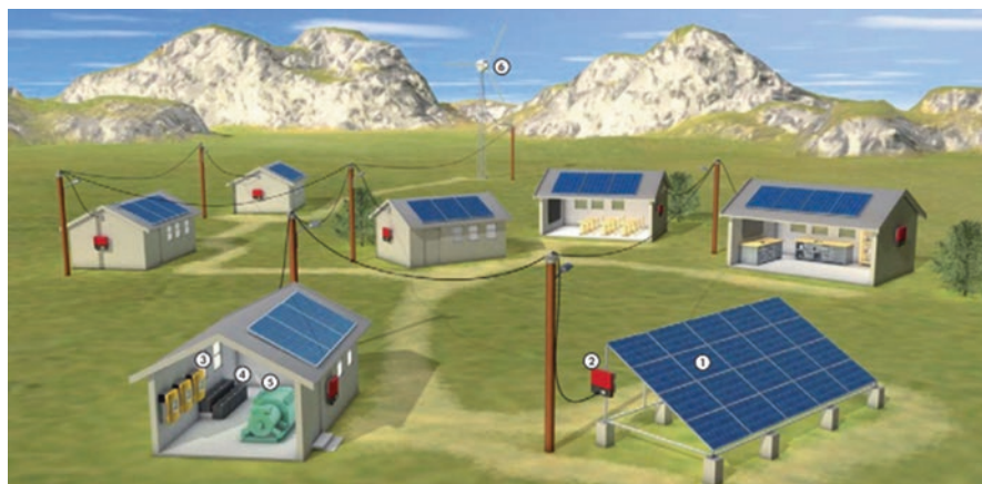
Fig. 8.3 An example of village solar/wind/diesel hybrid system. 1. PV generator, 2. PV inverter, 3. Battery inverter, 4. Storage battery, 5. Diesel generator, 6. Wind turbine. (Source: SMA 2010)
