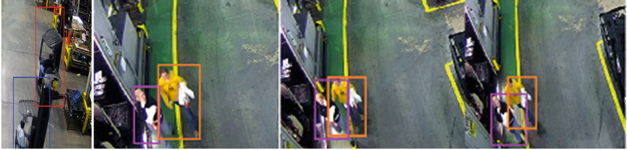
Fig. 3. Left. Occluded forklift tracking Right. Multiple occluded pedestrian tracking
