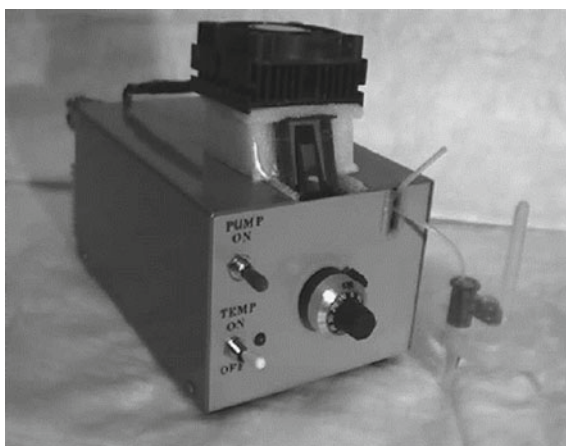
Fig. 8.5 SPR-system based on a texas instruments spretta with added temperature controller and peltier module for temperature regulation [16]
