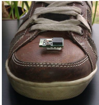
Fig. 9. Topview of the micro-IMU V3 which is mounted on a shoe [12].
