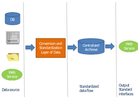
Fig. 6. Flow of collection, standardization, storage and access of the data [1].
