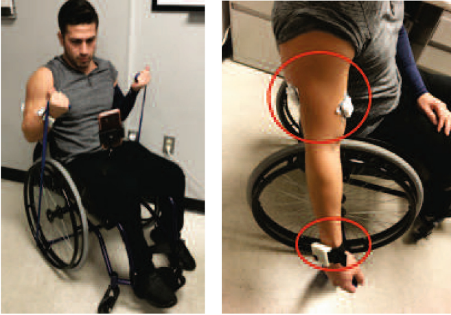
Fig. 2. Physical setup of the DREAM mobile fitness system. User dons wireless sensors (EMG Flexdots and custom IMU device) and exercises in wheelchair while monitoring progress on DREAM mobile app.
