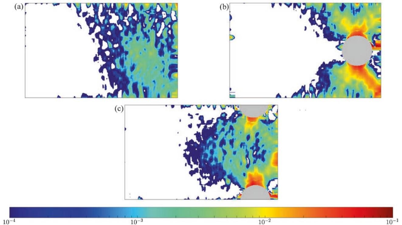
**Fig. 15.1** Typical longitudinal plastic strain at the last stage recorded during the IBII test (a) rectangular specimen, (b) specimen with a hole, (c) specimen with two notches
