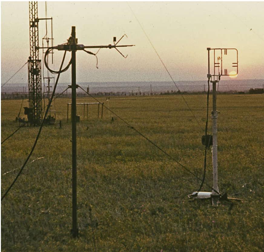
Fig. 26.1 Russian phase shift anemometer during the experiment ITCE-81(Tsvang et al. 1985) at the Tsymlyansk research area (left) together with the Japanese Kaijo-Denki sonic anemometer PAT 300, working with the travel time principle (Photograph: Foken)
