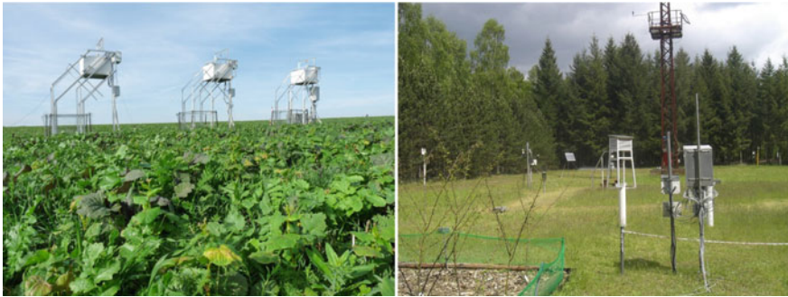
Fig. 5.12 Advanced technical systems for monitoring the status of soils and vegetation in agricultural landscapes. The left-hand photograph shows a gas-flux measurement station on cropland operated by the Thuringian State Institute of Agriculture, Germany. The station is combined with lysimeters. Researchers aim to understand processes of plant growth and cycles of water and fertilisers in soil, plant and ground-level air layer. The right-hand photograph shows part of forest measurement station operated by the Thünen Institute of Forest Ecosystems in Eberswalde, Germany
