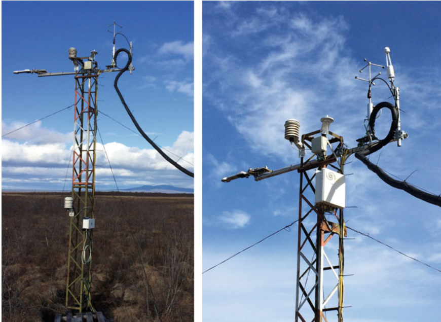
Fig. 26.4 Eddy-covariance tower at the Chersky research site (Photograph: Göckede). The system consists of a heated sonic anemometer (METEK USA1), an open-path gas analyzer for \text{CO}_2/\text{H}_2\text{O} (LiCor 7500, only right picture), and the inlet line for a closed-path gas analyzer for \text{CH}_4/\text{CO}_2/\text{H}_2\text{O} (Los Gatos FGGA)
