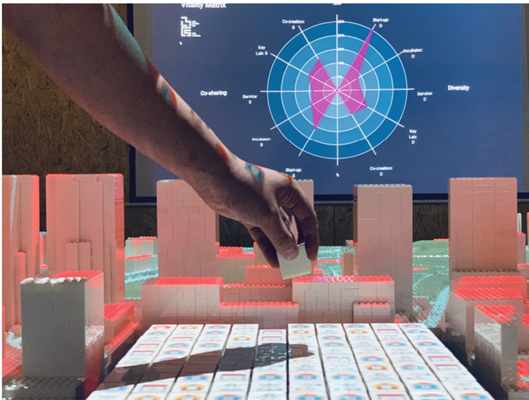
Fig. 1. The tangible user interface and simulation matrix of CSB. A user is manipulating a LEGO module to modify the distribution of entrepreneurial enterprises for community prototyping.
