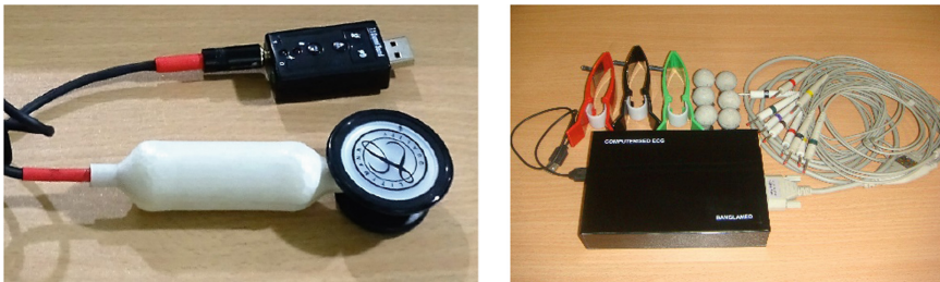
Fig. 3. Improved digital stethoscope (left) and indigenously designed and developed 12 lead diagnostic ECG device, which connects to a PC through USB port.
