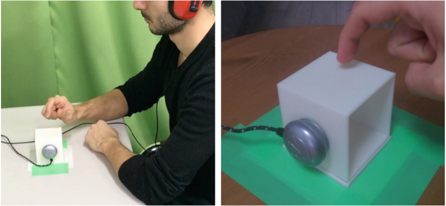
Fig. 5. Augmented sound experiment is designed by Lugtenberg et al. [18] for receiving a perception of thickness of an object differently when tapping it using two cubes (solid and hollow).
