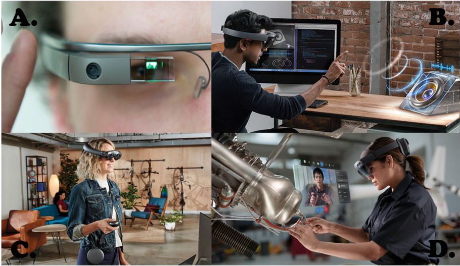
Fig. 3. Leading head-mounted wearable devices for AR from three companies. (A) is Google Glass, (B) is Microsoft HoloLens 1, (C) is MagicLeap One, and (D) is Microsoft HoloLens 2. (Image credit: http://time.com/ , https://news.microsoft.com/ , https://www.bloomberg.com/ and https://www.microsoft.com/en-us/hololens/buy )
