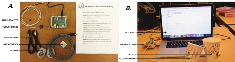
Fig. 4. (A) Exemplary toolkit using off the shelf parts. (B) a typical user case with the toolkit.
