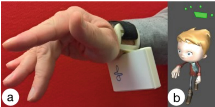
Fig. 4. A wrist-worn sensor, built and designed by Ens et al. [16], is used for controlling animations in the virtual world and designing mixed-scale gesture using a HoloLens augmented reality display.
