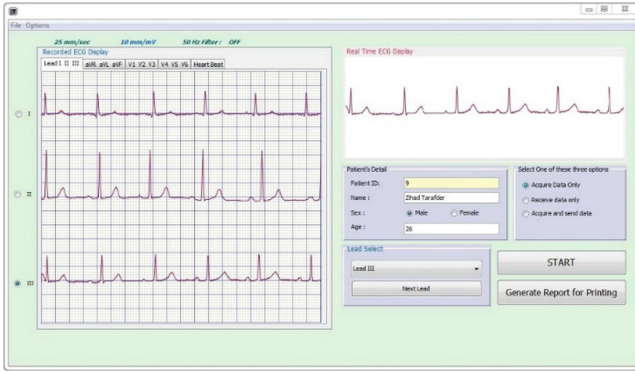
Fig. 4. Real time ECG display showing raw traces (top right window) and saved traces (left window). Patient information and data acquisition interface are also shown.
