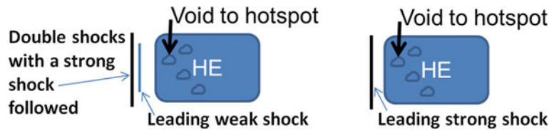
Fig. 39.1 Illustration of shock desensitization due to the hot-spot mechanism. Left sketch (first case in the text) has a weak leading shock followed by a strong shock, which has the same strength as the single leading shock of the right sketch (second case mentioned in the text). The vertical line stand for shocks travelling through the HE from left to right. The shorter vertical line represents the weak shock
