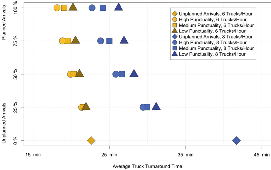
Fig. 1. Simulation model scenario analysis results in terms of average truck turnaround times, truck arrival punctuality, and percentage of planned arrivals (Color figure online)
