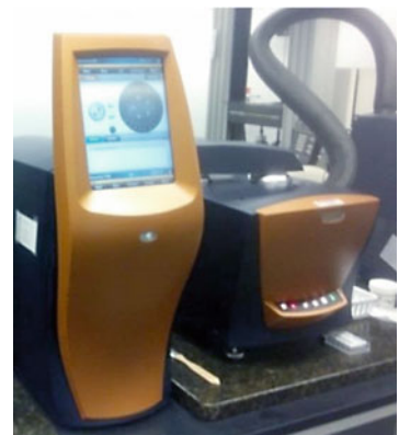
Fig. 1 (a) FlackTek DAC-600.1 VAC-P speed mixer, (b) Teflon molds for DMA and SHPB tests, (c) Polyurea samples for DMA and SHPB tests (the black samples have milled carbon fiber inclusions)
