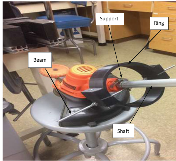
Fig. 1 Vibration absorber attenuation for the weed wacker
