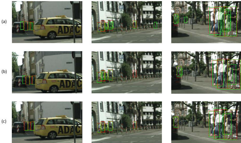
Fig. 6. The visualization of detection results. The first row((a)) displays the outputs of original ALFNet [11]. The second row((b)) displays the outputs of ALFNet with RFB. The third row((c)) displays the outputs of our proposed method. The green and red rectangles represent detection results and the ground truth results respectively. (Color figure online)
