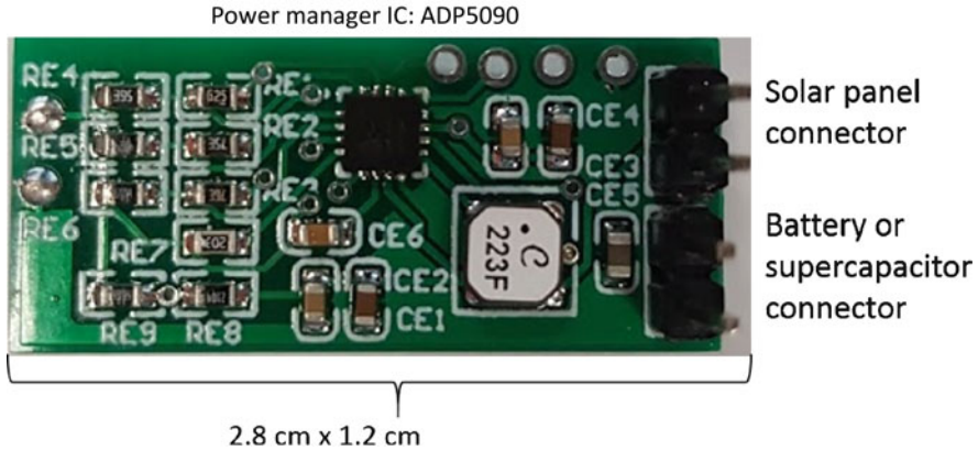
Fig. 15.2 Energy harvesting module
