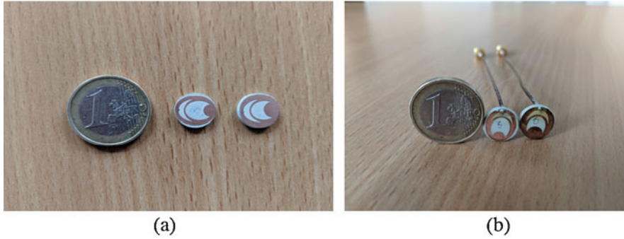
Fig. 40.4 Fabricated antennas (a) Antennas without coaxial cables. (b) Antennas with coaxial cable
