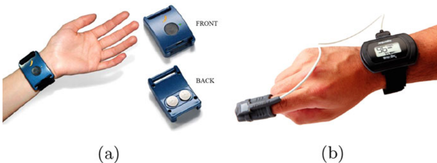
Fig. 32.1 (a) The wrist worn Affectiva records EDA, Acc, and Temp; (b) the Nonin 3150 Wireless WristOx2 records HR and SpO 2
