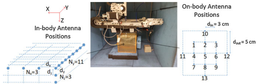
Fig. 39.5 Measurement setup and in-body and on-body positions for the channel modeling in lossy tissue
