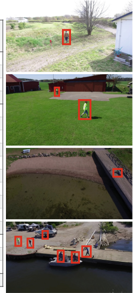
Fig. 4. Summary of video sequences and example images used for evaluation: four locations (T, M, V, K), different weather conditions and times of year, percentage size composition (small, medium, and large) and total number of objects of class person.
