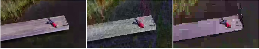
Fig. 2. Example frames from the evaluation sequence showing degradation of image quality when using different video encoding techniques with the same bitrate of 50 kbps. From the right: H.265, VP9, H.264.
