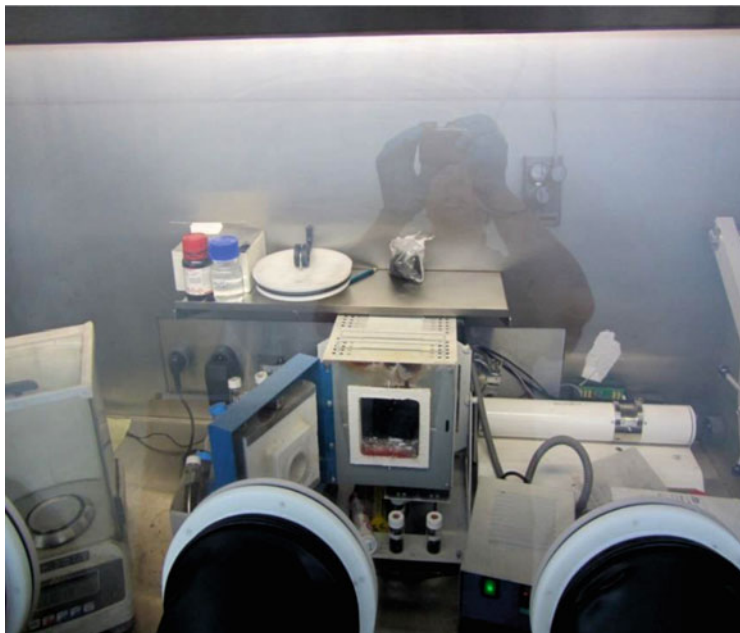
Fig. 8.2 A glove box with a furnace for the synthesis of sodium ferrate(IV). A room temperature Mössbauer spectrometer is installed directly inside the glove box (white tube on the right side)
