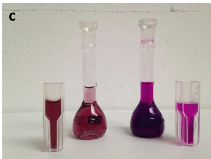
Fig. 13.6 (a) UV–VIS spectrum of ENVIFER 036 in aqueous solution at concentration 0.5 g/L. (b) UV–VIS spectrum of \text{KMnO}_4 in aqueous solution at concentration 0.5 g/L. (c) Differently colored aqueous solutions at concentration 0.5 g/L—commercial ferrate (on the left—pinkish and lighter) and potassium permanganate (on the right—purpler and darker)
