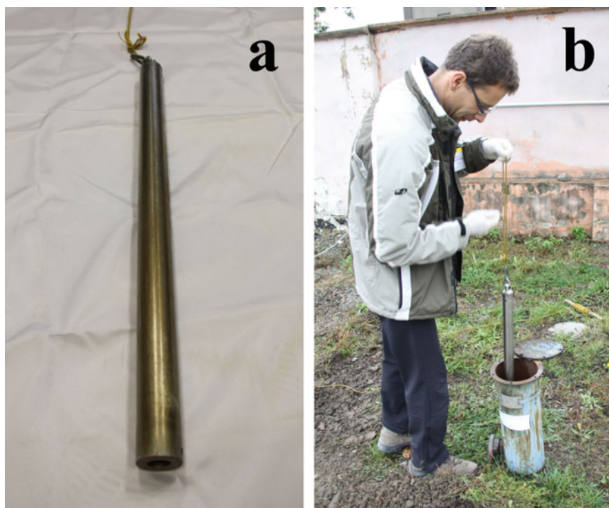
Fig. 33.3 Stainless steel bailer for sampling of groundwater and sediment in (a) a static mode and (b) its usage on site
