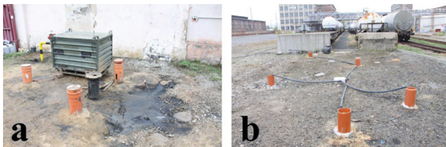
Fig. 33.5 Susceptibility measurement employing underground probes at (a) the Spolchemie Site I and (b) Spolchemie Site II
