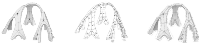
Fig. 8. Diagram showing the fabrication geometry (left), planes generated using Principal Component Analysis (center), result of PCA-based bounding box approach (right)
