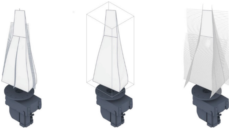
Fig. 9. Diagram showing the oriented component geometry (left), initial clustering of mesh faces based on HE connectivity (center), result of ruling generation based on subdivision of ordered mesh edges (right)
