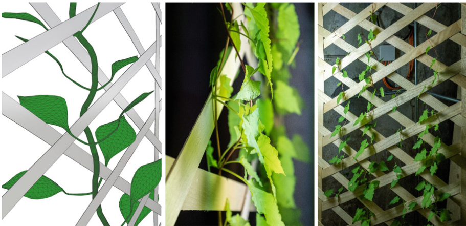
Fig. 3. Construction concept hypothesis with simulated bio-hybrid tri-axial weave (left), detail of hand-woven Fallopia interlaced with maple strips (centre), progression of Fallopia and spread of leaf cover (right)
