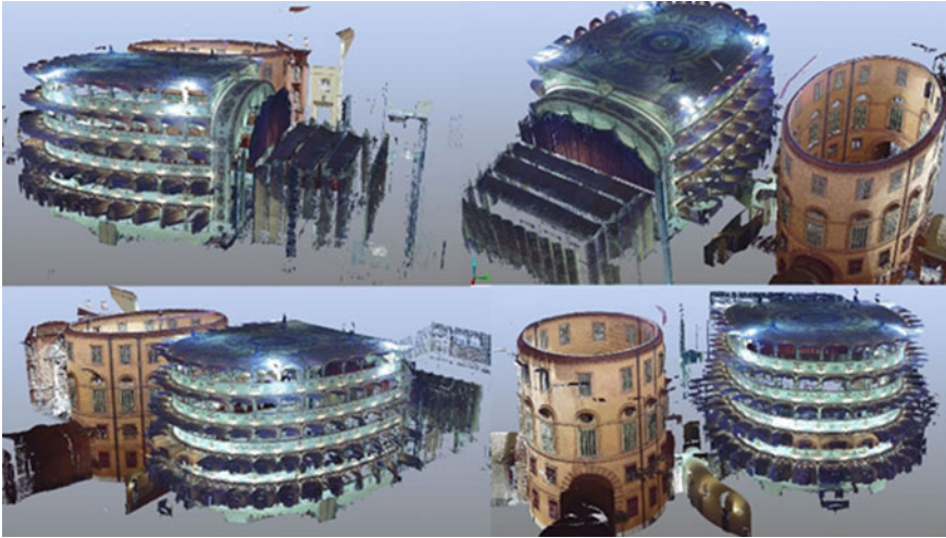
Fig. 2 Tridimensional point cloud of the inside of the theater and of Foschini's rotunda, obtained through a laserscan 3D Faro Cam 2 focus 3D survey. 9 scans were combined to obtain the complete cloud
