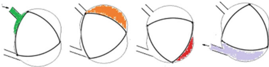
Fig. 8 The phases of the Wankel engine; in order: suction, compression, burst, discharge
