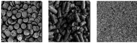
Fig. 2. PB25 in granular form, pellet form and powder form (from left to right).
