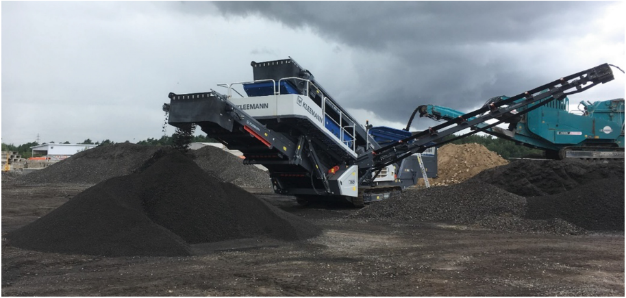
Fig. 2. Crushing and classifying (0/16, 16/22 and 22/x) of RAP in Lithuania
