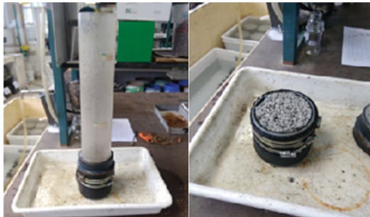
Fig. 2. Falling head permeameter device employed for the permeability test
