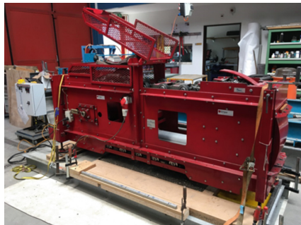
Fig. 9. Traffic Load Simulator MMLS3 situated on top of the constructed specimen
