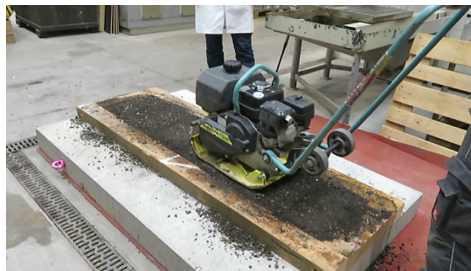
Fig. 7. Compaction of specimen for use with traffic simulator using a plate compactor
