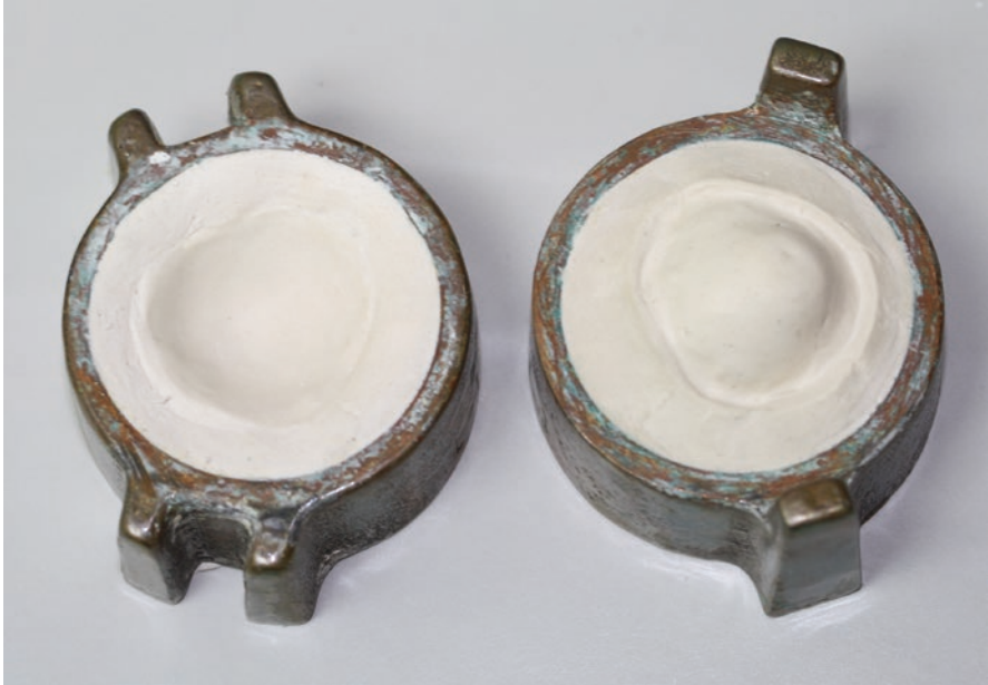
Fig. 22.7 The two-part mold is ready to be packed with clear PMMA dough. (Published with kind permission of Dr. Keith R. Pine. All rights reserved)
