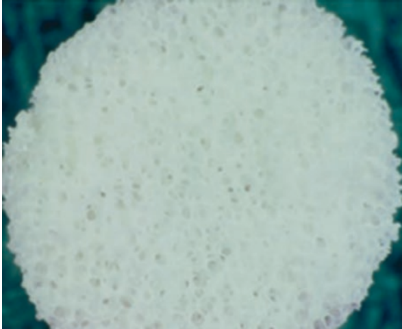
Fig. 5.9 A close-up view of an alumina orbital implant. (Image from Jordan and Klapper [28]. © Springer)
