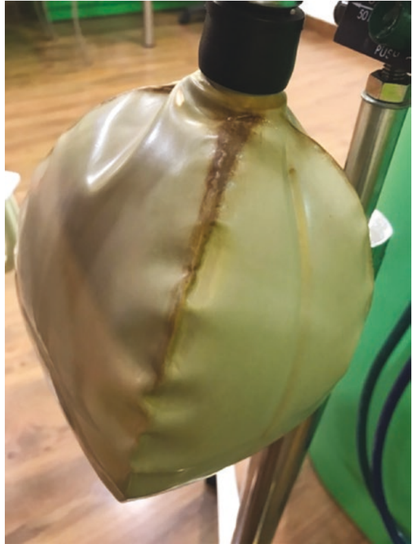
Fig. 6.12 Worn out reservoir bag with probable cracks causing leakage
