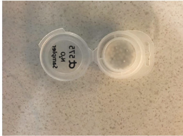
Fig. 6.4 Sampling holes in monitor badge
