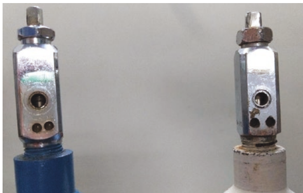
Fig. 4.25 Figure showing pin index system with nitrous oxide having two holes placed close to each other and oxygen having holes slightly apart
