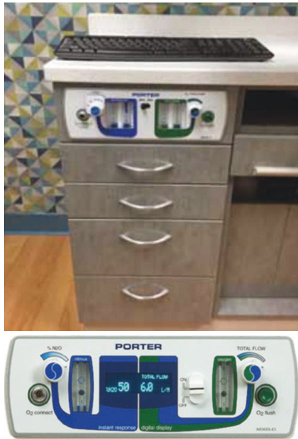
Fig. 4.20 Cupboard mounted flowmeter. (Source: http://www.porterinstrument.com/dentalcontent/files/datasheets/Porter-Full-Products-and-Accessories-Catalog-FM-1423.pdf )
