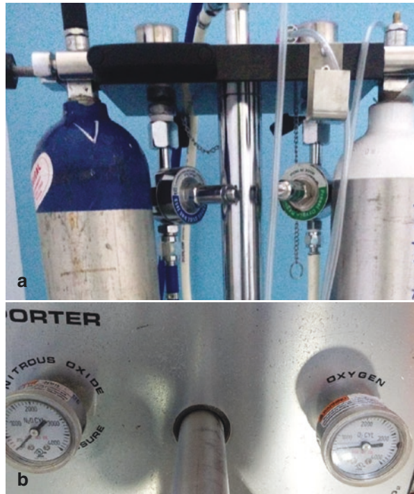
Fig. 4.15 (a) Figure showing regulators for nitrous oxide (blue) and oxygen (green) attached to the yoke; (b) pressure gauges for nitrous oxide and oxygen attached to yoke
