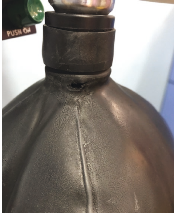
Fig. 6.11 Cracks and hole in reservoir bag
