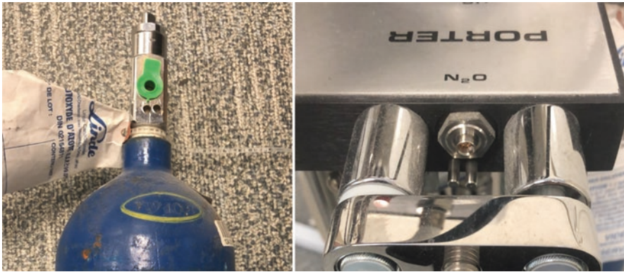
Fig. 2.9 Pin index system for nitrous oxide on cylinder and yoke of portable nitrous oxide delivery system
