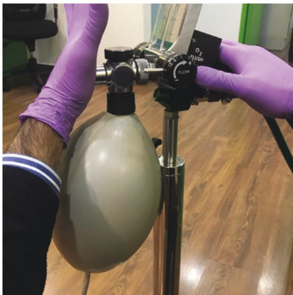
Fig. 4.30 (a) Figure showing failure of calibration check. (b) Figure showing properly calibrated flowmeter
