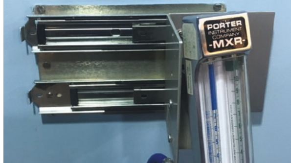
Fig. 4.21 Wall mount slide assembly for flowmeter
