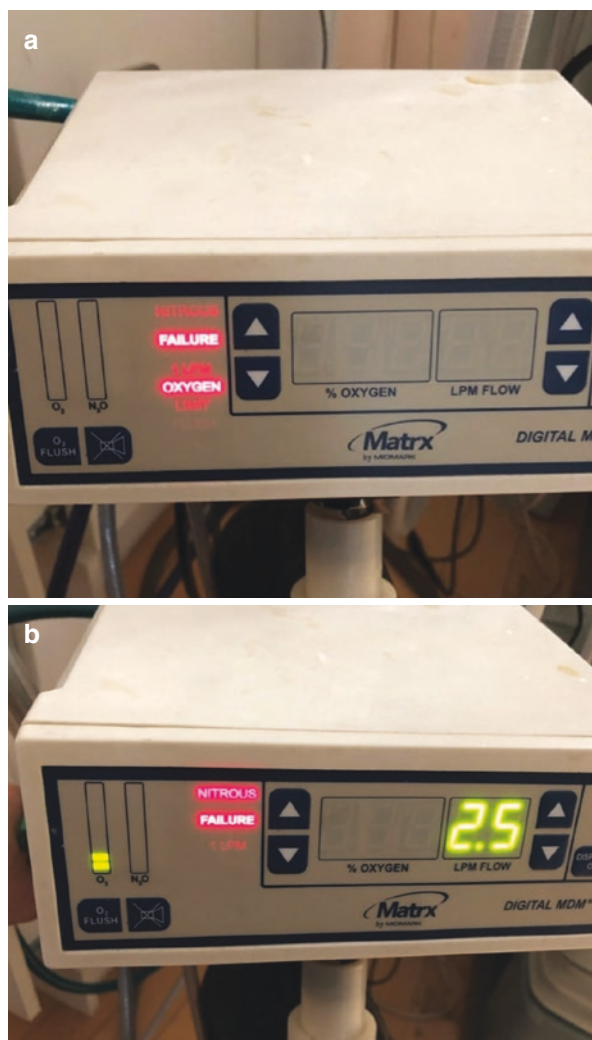
Fig. 4.29 (a) Figure showing reduction in line pressure of oxygen as failure oxygen which stops flow of nitrous oxide gas also due to fail safe mechanism. (b) Figure showing reduction in line pressure of nitrous oxide as nitrous failure . In this situation, oxygen flow continues as shown in this figure
