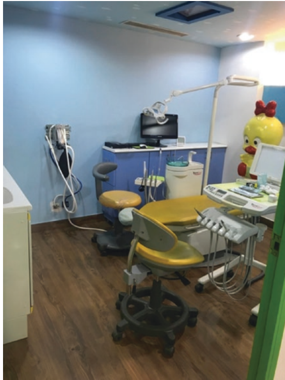
Fig. 6.18 A small-sized operatory with no windows can have higher concentrations of nitrous oxide in ambient air
