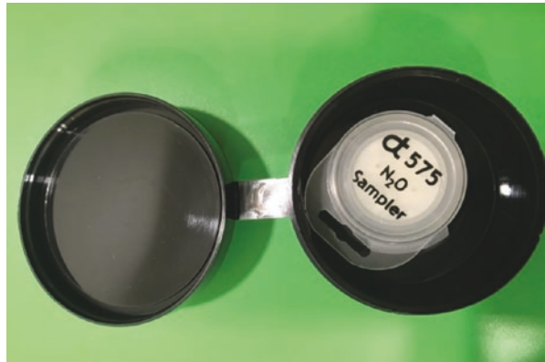
Fig. 6.7 Placing monitor in the air tight container after use, to be transported to the lab for analysis
