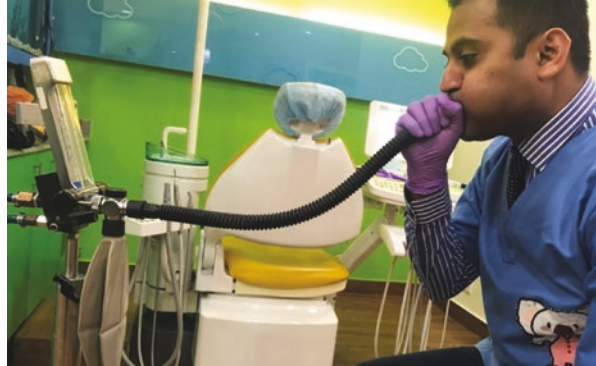
Fig. 4.32 Figure showing check for non-rebreathing valve. Reservoir bag does not inflate on blowing air into corrugated tube
