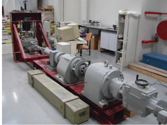
Fig. 8.46 Discontinuity shear tests at University of Porto
