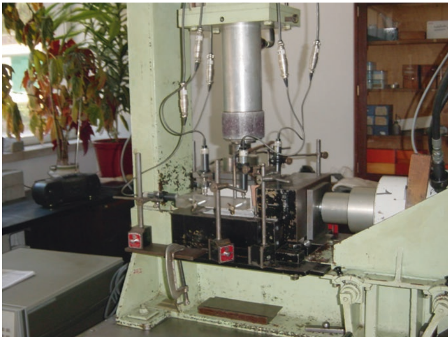
Fig. 8.45 Discontinuity shear tests at LNEC
