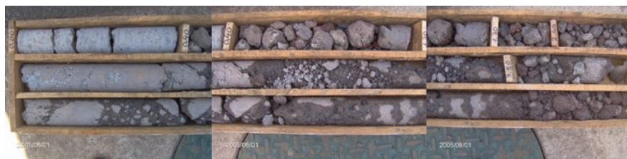
Fig. 20.10 Samples obtained in a borehole of the pumping station zone (Cafofo 2006)
