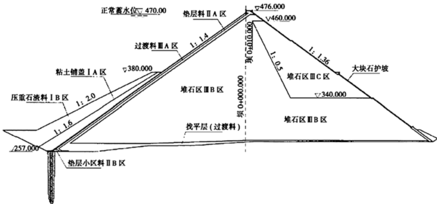
Fig. 25.18 Jiangpinche CFRD main cross section (Wang and OU 2013)
