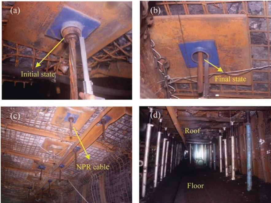
Fig. 17.24 (a–d) Roadway reinforcement effects using NPR support in a large buried depth coal seam
