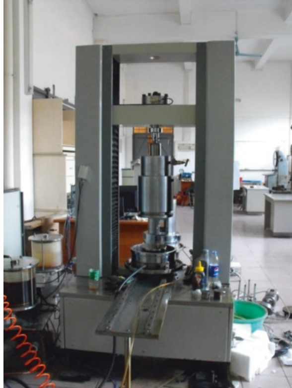
Fig. 8.22 Axial pressure loading system
