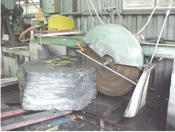
Photo 23.1 Saw with 1-m-diameter blade, used to reduce the size of the coal samples in the laboratory
