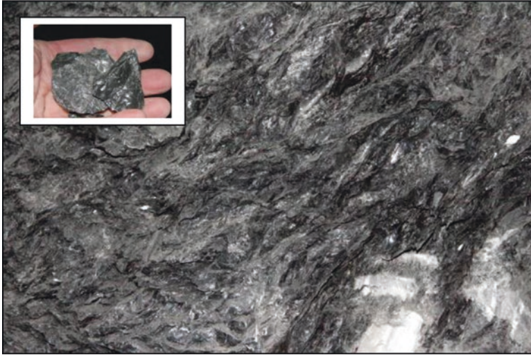
Fig. 19.7 Characteristic view of a sheared foliated intact rock, where it is extremely difficult to recover core of “intact” and representative rock elements and to prepare specimens for laboratory testing of the uniaxial compressive strength or point load test
