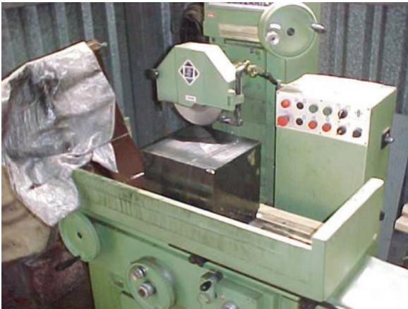
Photo 23.2 Flat-surface grinding used for finishing the cubic faces for load application
