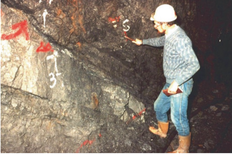
Fig. 8.16 Sandstone and siltstone sequence in a adit (Hoek 2007a)
