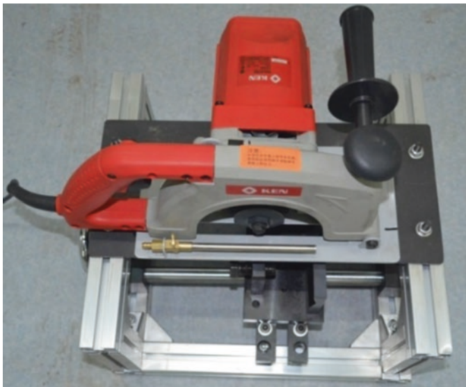
Fig. 7.18 Portable sample cutting machine (He et al. 2018)
