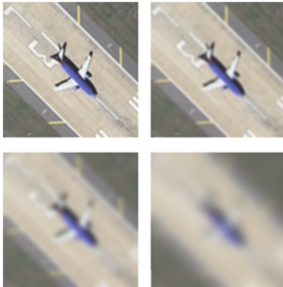
Fig. 6 Blurred images with different degrees of Gaussian blurring: \sigma = 0 (top left), \sigma = 2 (top right), \sigma = 5 (bottom left), and \sigma = 7 (bottom right)
