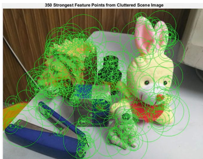
Fig. 7 Feature extraction of cluttered image taking 350 strong features
