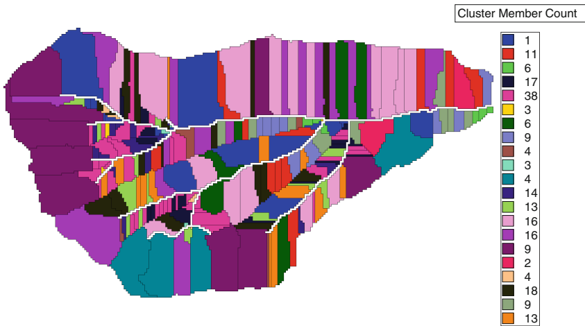
Fig. 7. Spatial distribution of K -means clusters at K = 37 applied on Wollefsbach catchment. All single member clusters are shown in dark blue. (Color figure online)
