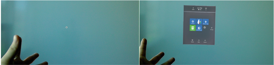
Fig. 4. Microsoft HoloLens can toggle between showing and hiding the main menu through a bloom gesture.
