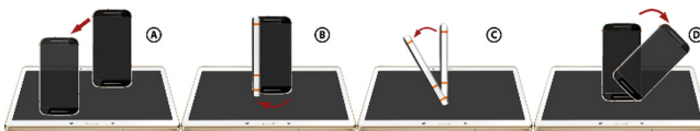
Fig. 3. Stacking physical gestures: (A) translation, (B) flat rotation, (C) tilt, and (D) corner rotation
