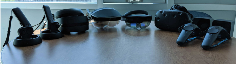
Fig. 5. Picture showcase a range of different HMD XR product. From left to right: HP windows mixed reality headset with inside-out tracked controllers, Meta 2 with built-in hand tracking, Microsoft HoloLens with gesture controls, HTC Vive with base station tracking. All these devices have differences that should be considered when designing for them.
