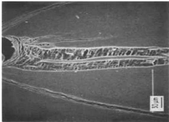
Fig. 5.22 Cold drawn behavior of a thermoplastic polymer up to failure
