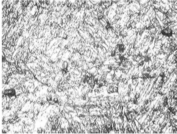
Fig. 4.38 Tempered martensite in steel. Metallographic microscope, Nital attack
