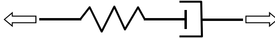
Fig. 5.14 Maxwell's model for glassy behavior; the strain is initially elastic, controlled by the spring, followed by viscous flow, controlled by the hydraulic dashpot
