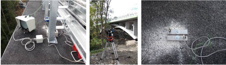
Fig. 4. The laser equipment and acceleration sensors used for dynamic testing.
