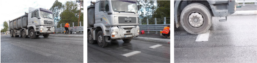
Fig. 7. Passage of the truck on a smooth roadway and through artificial unevenness of the surfacing reflected by a road bump.
