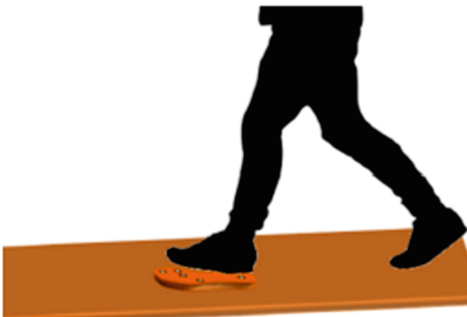
Fig. 8. Experimental setup for the proof-of-concept test with the instrumented insole acting as a fixed platform (adapted from [1]).
