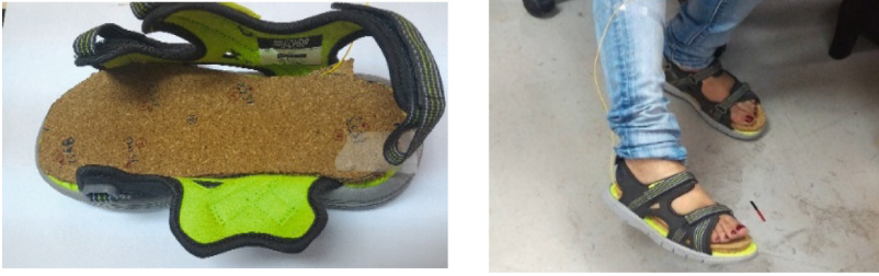
Fig. 10. FBG-embedded insole positioned inside a shoe for plantar pressure monitoring during the gait motion.
