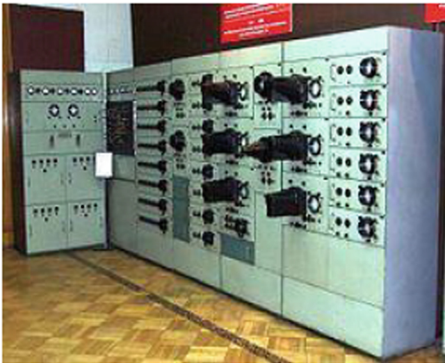
Fig. 2. Differential Equations Analyzer. Source: Archives of the Institute of Mathematical Machines with permission of the Institute’s director.
