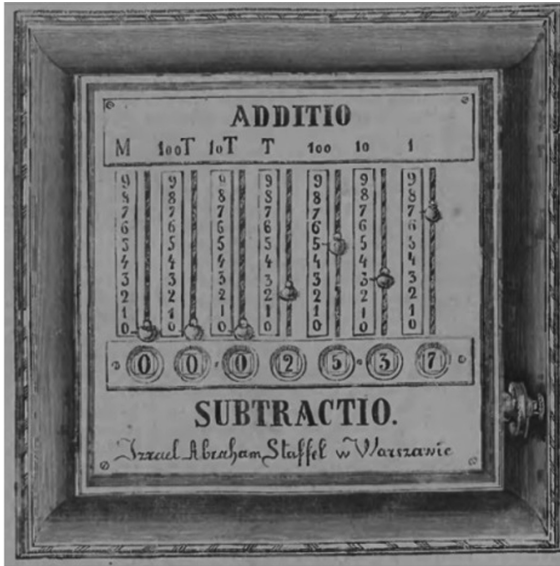
Fig. 4. Staffel's adding machine of 1858 [11].
