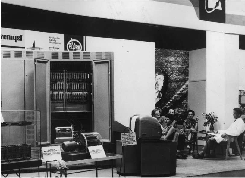
Fig. 9. UMC-1 at the exhibition in Moscow; drum memory was exposed in the foreground. Source: Polish Wikipedia
