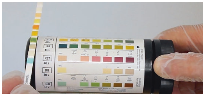
FIGURE 3.3 Urine reagent strip and manufacturer's chart. Used with permission from Siemens Healthcare Diagnostics Inc.
