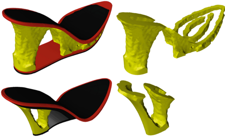
Fig. 5. Topological optimisation solutions for both shoes.
