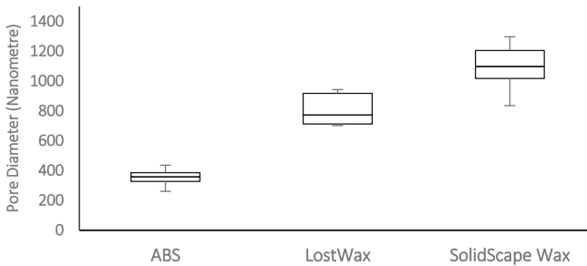
Fig. 1. Porosity of cellulose hydrogel by measuring internal pore radius of freeze-dried gel samples made with ABS, Lost wax and Solidscape™ wax molds.
