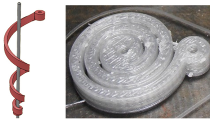
Fig. 4. Programmed part and AM coil in its flat form (Monzón et al. 2017)
