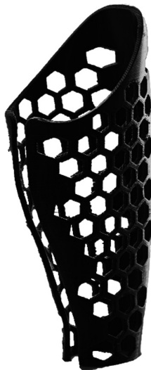
Fig. 5. The printed brace with hexagonal shape without any polishing.
