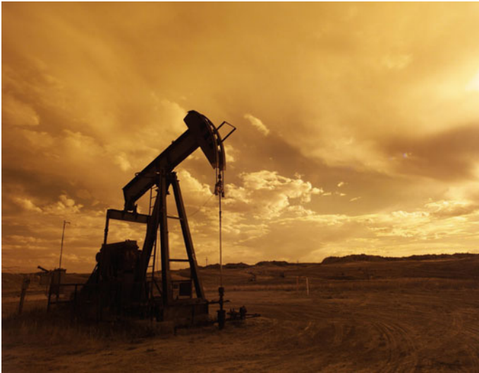
Fig. 4.4 A pumping jack in an oil field ( https://www.publicdomainpictures.net/en/viewimage.php?image=177469&picture=oil-pump-jack )
