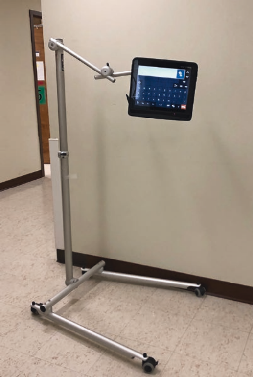
Fig. 34.3 Mounting system for communication device to ensure that the patient can access their AAC system across a range of physical positions
