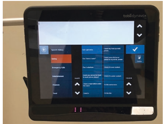
Fig. 34.2 Page set for eating-related vocabulary shown on a Tobii Dynavox i-15+ dedicated communication device. This device can be accessed by the patient using eye gaze, and scanning or through pointing with hands
