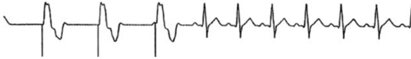
Fig. 10.7 Appropriate sensing inhibits the pacemaker when the intrinsic rate is above the pacing minimum rate
