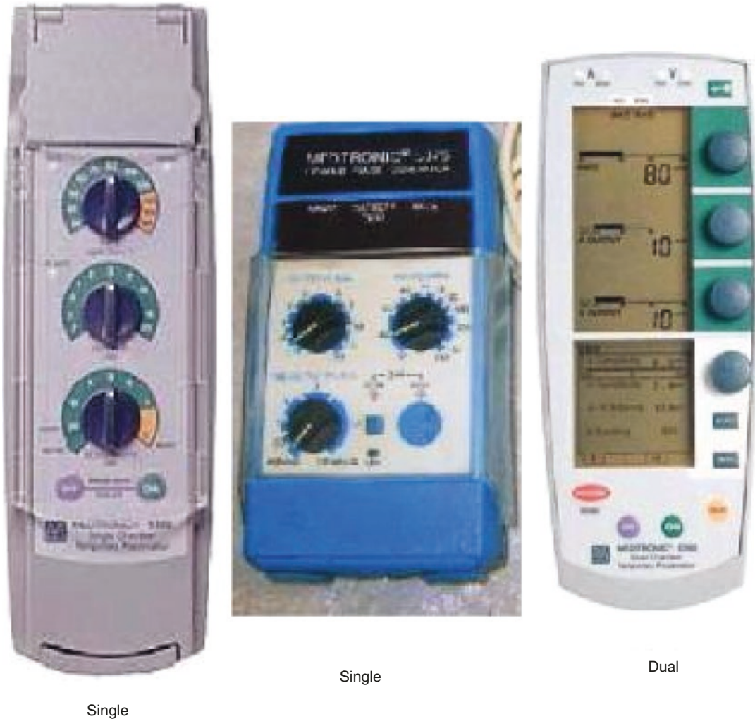
Fig. 10.13 Various models of pulse generators for transvenous or epicardial pacing
