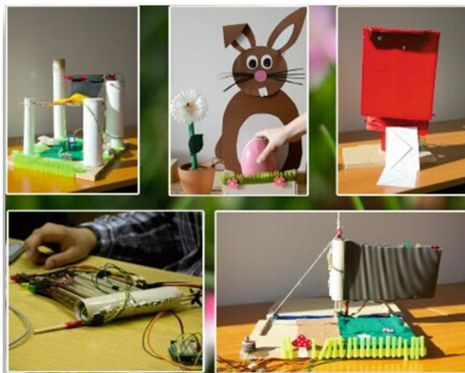
Fig. 3. Student results of physical computing: interactive objects with embedded systems.
