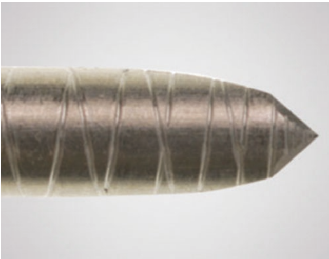
Fig. 10.9 Incision line on pickup needle to increase the echogenicity
