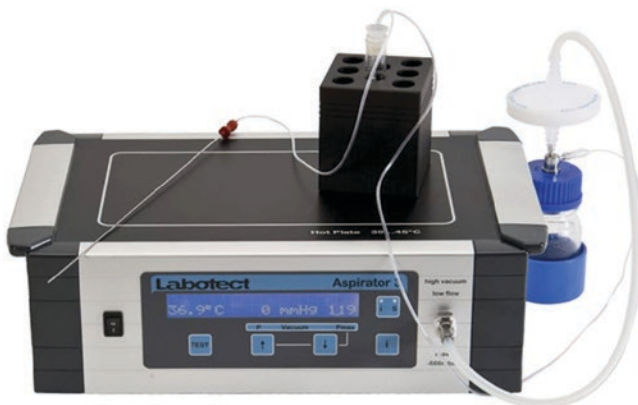
Fig. 10.21 Pump vacuum aspiration
