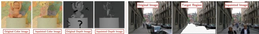
Fig. 2.3 Left: results of exemplar-based inpainting [36] applied to RGB and depth images. Note that the objective is to remove the object (baby) from both the RGB and depth images and to fill the already existing holes (pre-removal) in the depth image. The approach is significantly more effective when applied to colour images. Right: result of exemplar-based inpainting using an external database [60]
