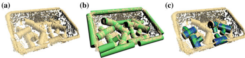
Fig. 13.9 Object detection based on geometric primitives [43]: a Point cloud captured by Cosero's Kinect camera; b Detected cylinders; c Detected objects
