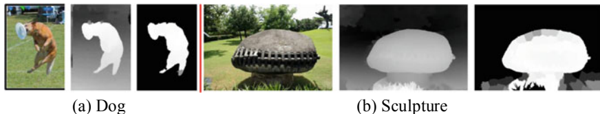
Fig. 10.7 Illustration of DSP descriptor. From the left to right in a group are the RGB image, depth map, and DSP map
