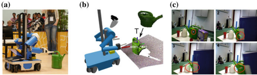
Fig. 13.10 Object tracking: a Cosero approaching a watering can; b A multi-view 3D model of the watering can (MRSMap, upper right) is registered with the current RGB-D frame to estimate its relative pose T , which is used to approach and grasp it; c Joint object detection and tracking using a particle filter, despite occlusion
