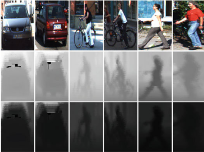
Fig. 17.5 In the first row, we have examples of cars, cyclists, and pedestrians as seen by a monocular camera. The second and third lines show the corresponding DMs generated from LIDAR data using Bilateral filter, with mask size of 13 \times 13 , and 8-bit linear and inverse range encoding, respectively
