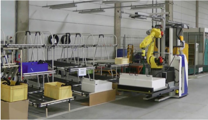
Fig. 13.15 The STAMINA cognitive robot performing an industrial kitting task in the experimental kitting zone at PSA Peugeot Citroën
