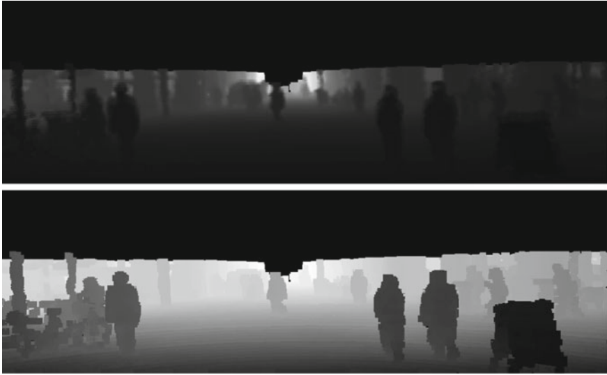
Fig. 17.4 Depth-map using the Bilateral filter with mask size 13 \times 13 . In the first row, the DM was generated using range-linear quantization while, in the second row, range-inverse was used instead
