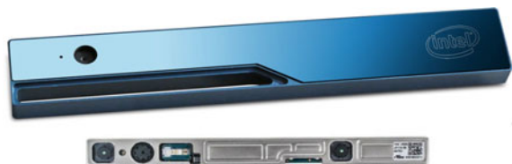
Fig. 14.2 The RealSense R200 sensor by Intel (from https://www.intel.it/ )
