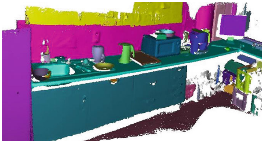
Fig. 6.6 Illustration of results from semantic RGB-D SLAM. Different colors indicate different object categories. Figures taken from [111]
