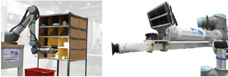
Fig. 13.18 Our system at the Amazon Picking Challenge 2016. Left: Full system including robotic arm, endeffector, shelf, and red tote. Right: Custom-built endeffector with linear and rotatory joints, two Intel RealSense SR300 RGB-D cameras, and lighting
