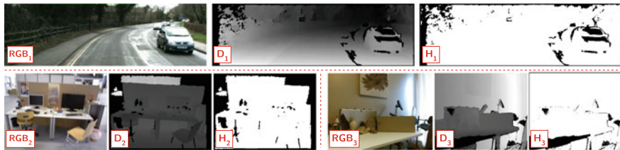
Fig. 2.1 Examples of depth acquired via stereo correspondence (top), structured light device (bottom left) and time-of-flight camera (bottom right). RGB : colour image; D : depth image; H : hole mask indication missing depth values
