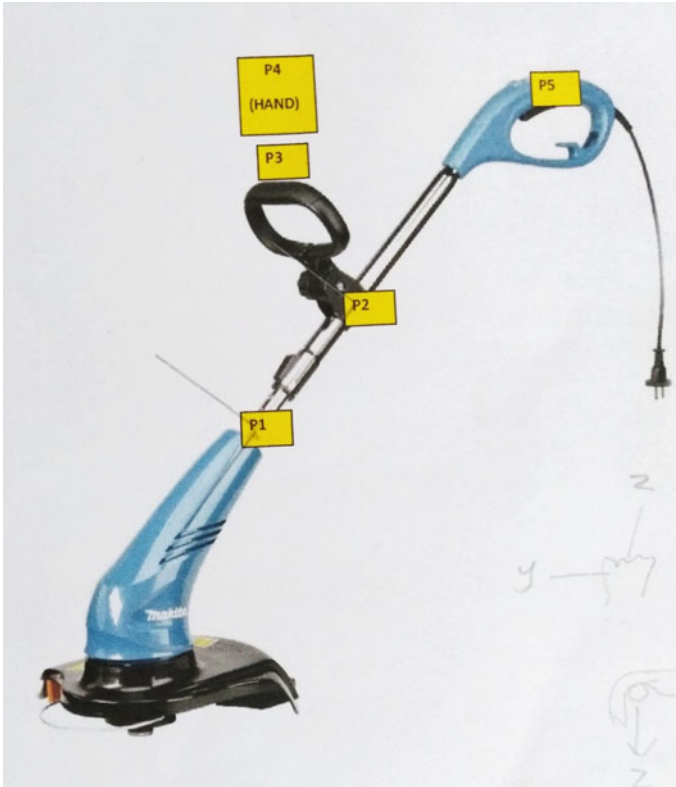
Fig. 1 Measurement points of the electric grass trimmer
