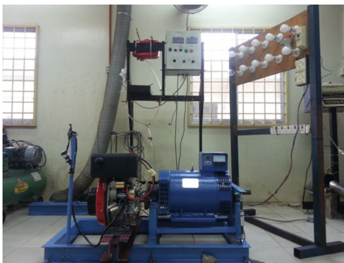
Fig. 2 Yanmar 178F diesel engine coupled with engine dynamometer
