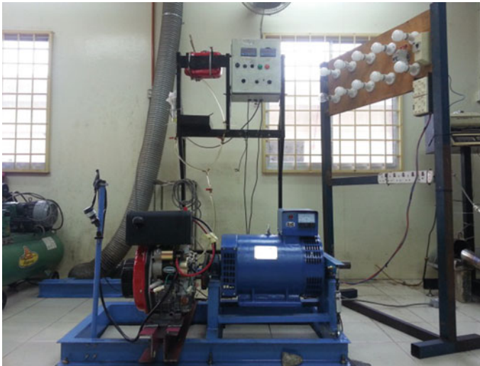
Fig. 1 Yanmar 178F CI engine performance experimental setup
