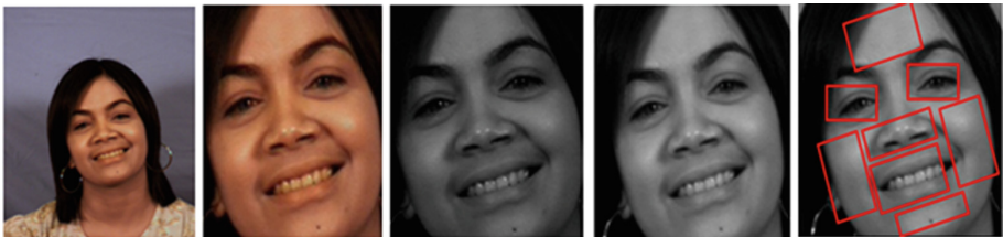
Fig. 2. (a) Original image (b) Face detection (c) Gray scale (d) Histogram equalization (e) Detected the components
