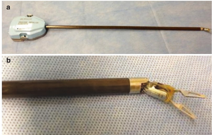
Fig. 2.26 (a) Da Vinci® robot precise bipolar forceps. (b) Tip of Da Vinci® robot precise bipolar forceps
