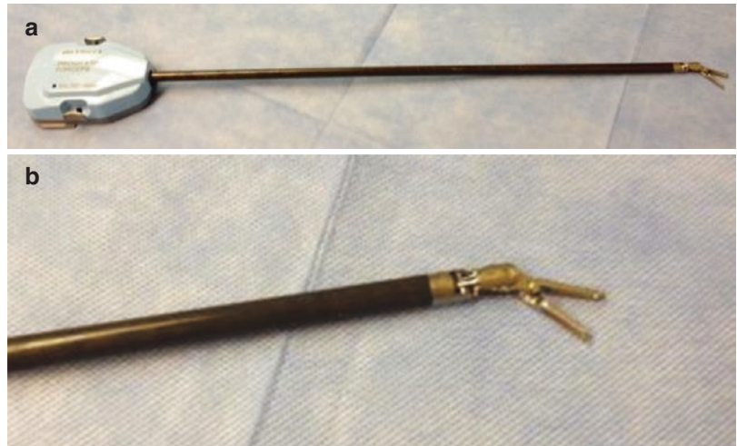
Fig. 2.27 (a) Da Vinci® robot prograsp forceps. (b) Tip of Da Vinci® robot prograsp forceps
